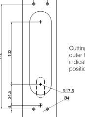
Cutting Prep to fit to outer face. Dashed lines indicate panic exit position (34.5 & 6).
