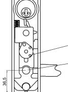
Ensure operating dowel is engaged in slot.
