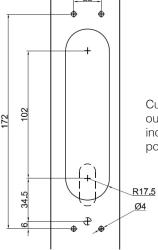
Cutting Prep to fit to outer face. Dashed lines indicate panic exit position (34.5 & 6).
