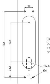
Cutting Prep to fit to outer face. Dashed lines indicate panic exit position (34.5 & 6).
