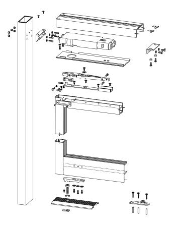
The Axim TC9900 Series – Market leading through durability, an Axim concealed closer is a hidden closing solution held integrally in the door leaf and transom. This means that the door requires no external hardware creating an aesthetically pleasing solution. The correct closing solution is dependent on the door and configuration. Also available fully adjustable, sizes 1 to 4
