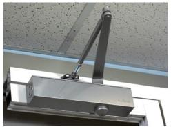
The FC-1500 is a multi-strength surface mounted hydraulic door closer, designed to complement the FC-1000. A hardened rack and pinion mechanism is housed in a die cast aluminium body.
