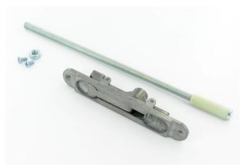
Flush door bolts are rebated into a door, and are normally operated by a small lever which sits perfectly flush both when the bolt is engaged and the doors closed. For maximum security Axim flush bolts have a hardened steel bolt, zinc plated with an anti-rattle sleeve and secure the slave leaf of a pair of doors. A standard installation requires two flushbolts morticed into the top and bottom of the door.
