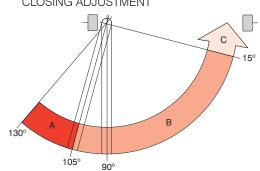
Independent valve screws permit closing speed adjustment from fully open to 15° and 15° to closed.
