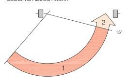
Independent valve screws permit closing speed adjustment from fully open to 15° and 15° to closed.
