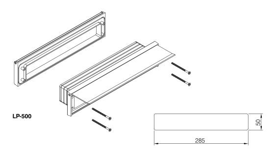
Rail preparation: 285 x 50mm cut out \*No fixing holes necessary\*
