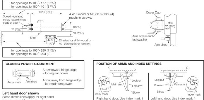
Same dimensions apply for right hand door measured from hinge edge.
